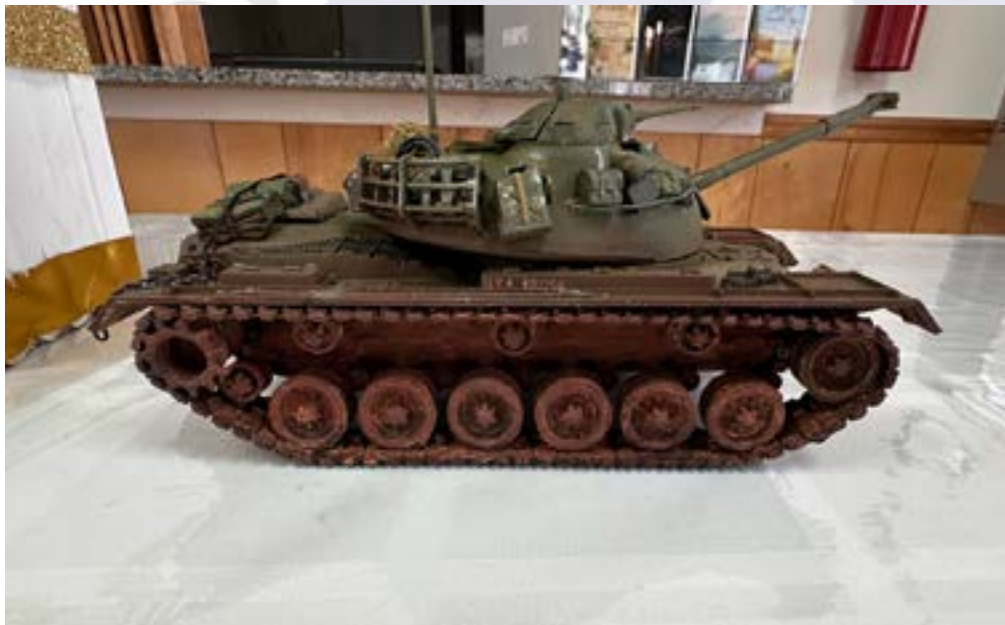
(left) Robert Bracken took a break from his normal figure painting to assemble this fine armored vehicle. In Robert's words: "The Monogram Patton tank was fun to build. I weathered the model as if it was in the Vietnam war. I airbrushed in Mig one shot green. Then weathered. I added water based putty mix with gravel to give the red clay look on wheels and track."
